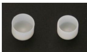
Figure 6: Mössbauer sample holder, bottom (left) and top (right).
